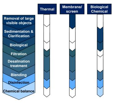
Most sub-processes in these sectors involve membrane, chemical and/or thermal treatment, depending on the technical characteristics, quality of the input/output, and/or cost.
