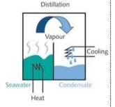
Vaporizing water, then condensing it, leaves some dissolved molecules/matter behind. This process is used in desalination to produce freshwater by vaporizing saline feedwater.
