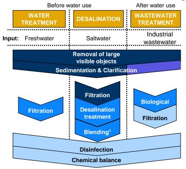
The wastewater treatment and desalination value chains consist of the same processes (sedimentation, filtration, disinfection etc..) as water treatment with specific additional processes (respectively, biologically activated sludge treatments, and desalination plus blending).
