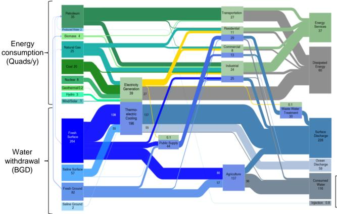
U.S. thermoelectric cooling withdraws the largest volume of water, and the petroleum sector (including frac'ing) represents a small fraction of U.S. water consumption
